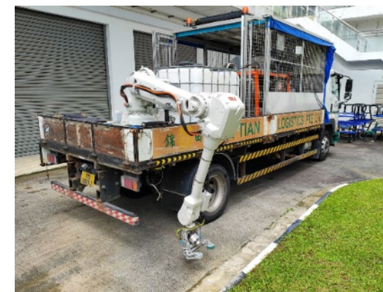
Automated Kerb Maintenance
